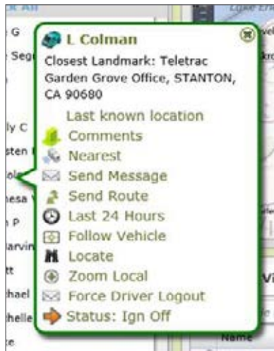
Right-click on a vehicle name or a data point to use the pop-up action menu options, including the Send Message feature.
